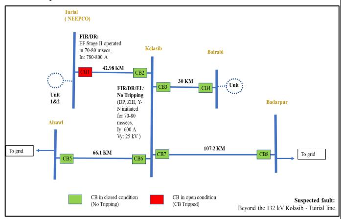
The 132 kV Kolasib-Tuirial line tripped at the Tuirial end on operation of Backup Earth Fault (EF) Stage II within 70–80 milliseconds, with a neutral current (In) of 780–800 A in all three instances.
