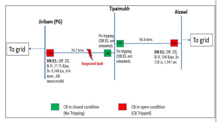
For 132 kV Aizawl - Tipaimukh Line: High resistive fault of slowly growing fault current cleared by the Main protection in DP, ZII, B-E. Total fault duration is of 1047 msecs.
