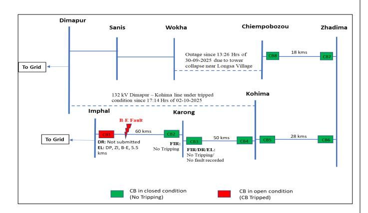
At 17:16 Hrs on 02.10.2025, 132kV Dimapur - Kohima tripped at Kohima end on B-Phase, Z-1.
