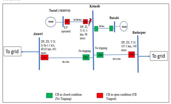
As per DR analysis, Y-N fault (Iy-1.1 kA, In-1.1 kA) initiated at 15:51:25.738 Hrs which was cleared within 405 msec from Aizawl end on operation of DP, ZII and within 546 msec from Badarpur end on operation of DP, ZII. There was no tripping from Kolasib end.
