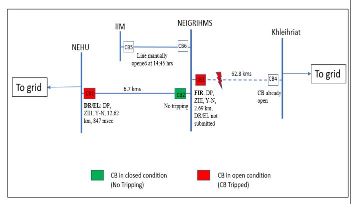
As per DR analysis, at 14:27:26.076 Hrs, R-Y-B fault started in 132 kV NEIGRIHMS-Khleihriat line which was cleared within 582 msec from Khleihriat end on operation of DP, ZII. Fault cleared within 65 msec from NEIGRIHMS end on operation of DP, ZI. Ir-3.9 kA, Iy-4.07 kA, Ib-4.16 kA.
