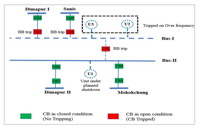
As per DR analysis of 132 kV Doyang-Dimapur I line, R-B (Ir=1.04kA, Ib=0.9kA) fault initiated at 19:59:32.761 Hrs. Fault was cleared within 52 msec from Doyang end on operation of Bus bar Trip. Also, Z5(rev) started at 19:59:32.786 Hrs.
