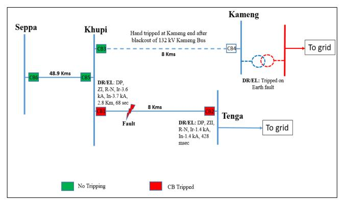
As per DR analysis, R-N fault (Ir-3.6 kA, In-3.7 kA) in 132 kV Tenga-Khupi line at a distance of 2.8 Km from Khupi initiated at 18:18:13.361 Hrs and cleared within 68 msec from Khupi end on operation of DP, ZI. Fault cleared within 428 msec from Tenga end on ZII.
