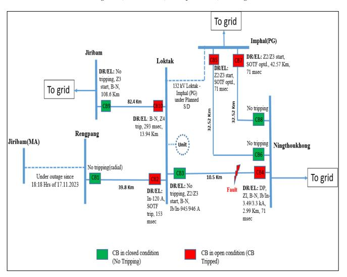
As per DR analysis, resistive B-N fault (Ib-3.49 kA, In-3.3 kA) in 132 kV Loktak-Ningthoukhong line at a distance of 2.99 Km initiated at 11:38:07.129 Hrs which was cleared within 71 msec from Ningthoukhong end on operation of DP, ZI. ZII started at Loktak end (no tripping) and fault current disappeared within 293 msec. 132 kV Loktak-Jiribam line tripped from Loktak end on Z4 within 293 msec (FD: 13.94 Km). Z3 start from Jiribam end and no tripping.
