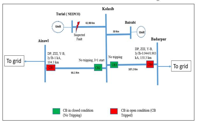
As per DR analysis, Y-B phase fault with Iy-1 kA, Ib-1 kA initiated at 14:24:10.766 Hrs which was cleared from Aizawl end within 861 msec and from Badarpur end within 853 msec on operation of DP, ZIII. There was no tripping from Kolasib end for both the lines.
