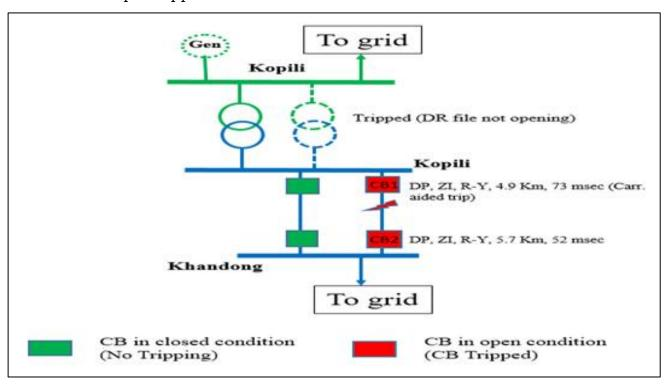
As per DR analysis, R-Y phase fault (Ir-3.2 kA, Iy-3.3 kA) in 132 kV Khandong-Kopili I line initiated at 13:53:51.371 Hrs and cleared within 52 msec on operation of DP, ZI from Khandong end. At Kopili end, fault cleared within 73 msec on operation of DP, ZI (Carrier aided tripping).
