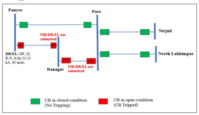
As per DR analysis, R-N fault (Ir-22 kA, In-23 kA) initiated at 18:10:13.739 Hrs which was cleared within 83 msec from Panyor end on operation of DP, ZI.
