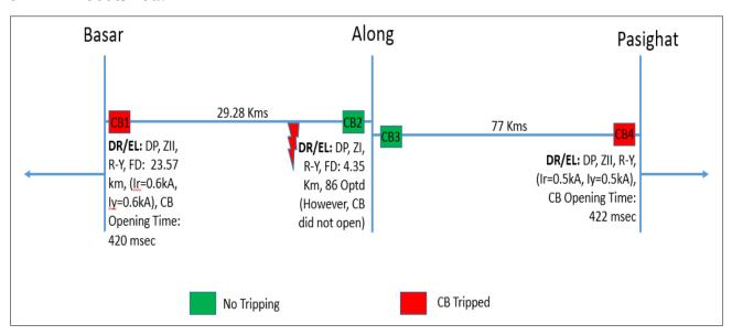
As per DR analysis, high resistive R-Y fault (Ir-697 A, Iy-683 A) in 132 kV Along-Basar line initiated at 00:39:00.712 Hrs which was cleared within 420 msec from Basar end on operation of DP, ZII, R-Y, FD: 23.57 km. ZI started from Along end and trip command issued. However, CB at Along fails to open. Non-isolation of fault
