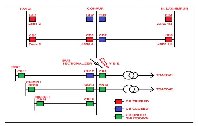
To address the issue with CB12 of BNC feeder, the CB was attempted to be opened but operation was unsuccessful. As a result, to isolate the CB of BNC bay, a shutdown of the bus section connected to BNC bay was availed.
