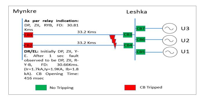
As per detailed report submitted by MePGCL, the 132kV link line from the 11kV/132kV Transformer Bay to the Switchyard passes through forest. Fault may have occurred in this line which is protected by O/C E/F relay.
