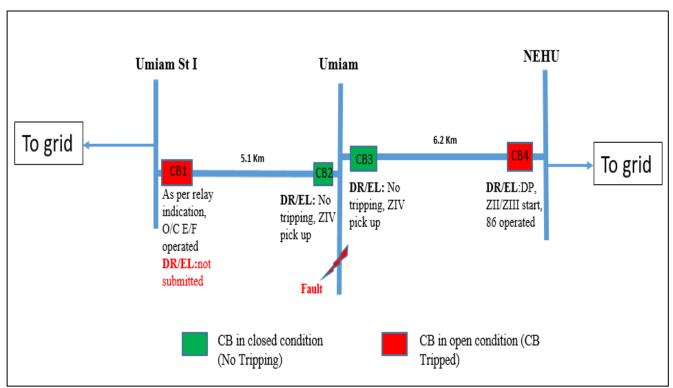
As per DR analysis, R-N fault (Ir-3.1 kA, In-2.9 kA) initiated at 01:55:31.117 Hrs which was cleared within 121 msec from NEHU end. ZII/ZIII start and 86 operated at 01:55:31.202 Hrs. Z4 pickup at Umiam end (no tripping).
