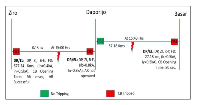
As per DR analysis, B-phase to E fault occurred in 132 kV Ziro-Daporijo Line at 15:00:13.363 Hrs and fault was cleared from Ziro on Z-1 within 57 msec, A/R successfully operated and Daporijo on Z-1 within 56 msec, A/R not attempted. At 15:43:18.118 Hrs, another R-Y fault occurred in 132 kV Basar-Daporijo line and fault was cleared from Basar on Z-1 operation within 80 msec. There was no\_tripping from Daporijo as radially connected.
