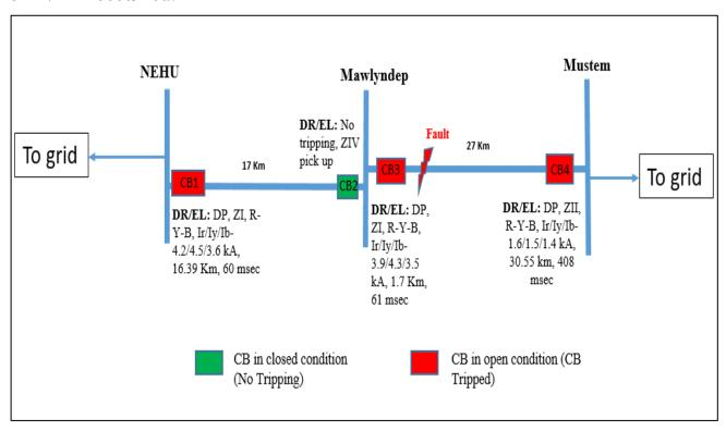
As per DR analysis, R-Y-B fault in 132 kV Mustem-Mawlyndep line with Ir-1.6 kA, Iy-1.5 kA, Ib-1.4 kA initiated at 12:06:38.585 Hrs and cleared within 408 msec on operation of DP, ZII (fault distance- 30.55 Km) from Mustem end. Fault cleared within 61 msec from Mawlyndep on ZI. Carrier was send from Mawlyndep end. However, Mustem CB tripped after ZII time delay.
