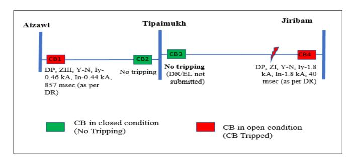
As per DR analysis, Y-N fault in 132 kV Jiribam-Tipaimukh line cleared within 40 msec from Jiribam end on operation of DP, ZI. Carrier signal was sent to Tipaimukh end from Jiribam. However, CB at Tipaimukh end did not trip until 800 msec from inception of fault which led to clearing of fault by tripping of healthy 132 kV Aizawl-Tipaimukh line from Aizawl end on operation of DP, ZIII within 857 msec.
