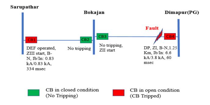
As per DR analysis, B-N fault was in 132 kV Dimpaur-Bokajan line with Ib:6.6 kA, In:6.8 kA, Vbe:32 kV and cleared from Dimapur on Z-1 within 60 msec. At Bokajan end, Z-2 pickup.
