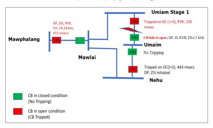
As per DR analysis of Umiam end of 132 KV Umiam Stage 1- Umiam, R-Y-B (Ir-Iy-Ib-2.5 kA) phase fault initiated at 13:35.32.800 Hrs. Distance Protection detected the fault in ZI and Trip command issued. However, CB fails to open at Umaim resulted in the opening of CB at Nehu for 132 KV NEHU – Umiam.
