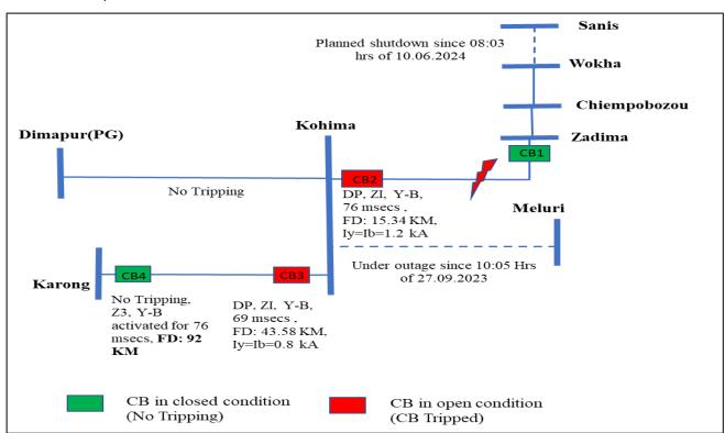
At 22:30 Hrs, Y-B fault occurred in 132 kV Kohima- Zhadima line as confirmed from the DR of **CB2** showing ZI (tripping) & CB4 showing ZIII (no tripping).
