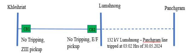
As per DR analysis of Khliehriat end, solid R-Y-B fault (Ir-2.2 kA, Iy-2.4 kA, Ib-2,4 kA) initiated at 06:38:48.098 Hrs and fault current disappeared within 64 msec. Again, at 06:38:48.322 Hrs, Y-E fault (Iy-1.5 kA, In-1.3 kA) reappeared and fault current disappeared within 471 msec. **DP, ZIII** pickup at Khliehriat end. There was no tripping from Khleihriat end.
