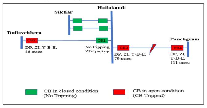
As per DR analysis, Y-B-E fault (Iy-8.3 kA, Ib-7.3 kA, In-2.6 kA) in 132 kV Hailakandi-Panchgram line cleared within 79 msec from Hailakandi end on DP, ZI & 111 msec from Panchgram end on DP, ZI.
