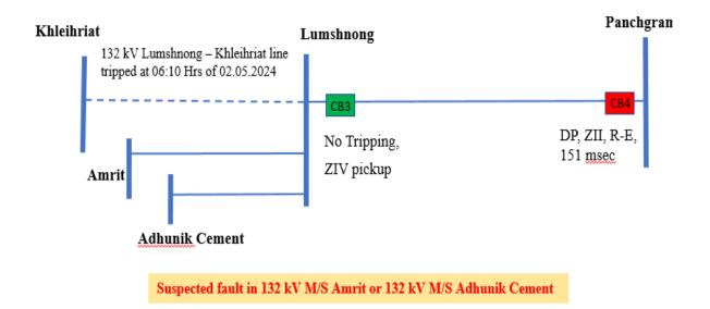
As per DR analysis, R-E fault (Ir-1.8 kA, In-1.4 kA) initiated at 07:00:11.821 Hrs in 132 kV Lumshnong-Panchgram line cleared within 151 msec on operation of DP, ZII from Panchgram end only. ZIV start at Lumshnong end which inferred that fault is in reverse direction.
