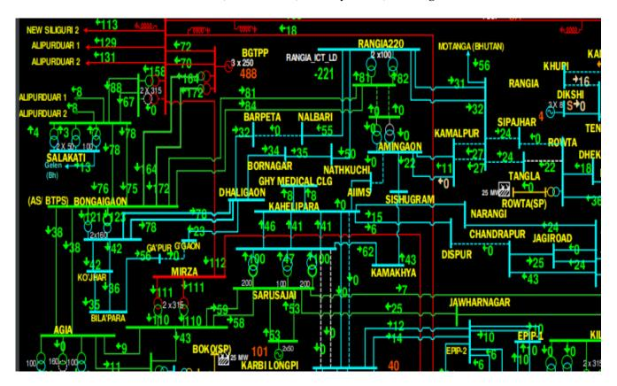
As per the analysis, there was no fault on the system at the time of event. As such tripping of all elements on LBB protection inferred to be UNWANTED. AEGCL is requested to update the root cause of maloperation of LBB/Bus bar protection and its corrective actions taken to avoid repetition.
