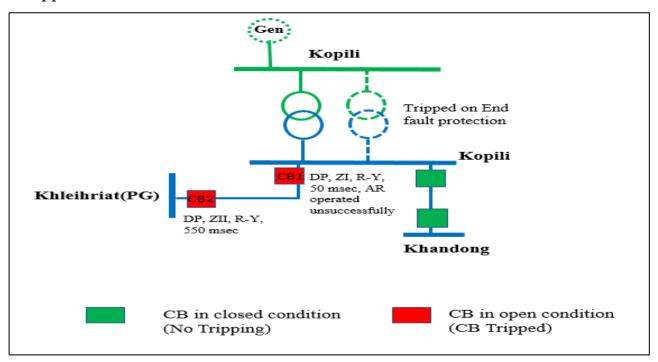
As per DR analysis of 132 kV Kopili - Khleihriat line, R-Y fault (Ir-6.5 kA, Iy-6.5 kA) cleared within 50 msecs on operation of DP, ZI from Kopili end and within 550 msec from Khleihriat end on operation of DP, ZII (As reported by POWERGRID, the line tripped due to falling of tree on line at span no. 21 to 22).
