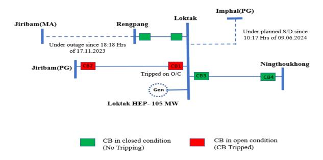
At 10:32 Hrs of 09-06-2024, 132 kV Loktak-Jiribam(PG) line tripped from Loktak end on Overcurrent due to which 132 kV Loktak-Ningthoukhong line got overloaded and subsequently all three units of Loktak tripped leading to generation loss of 105 MW.
