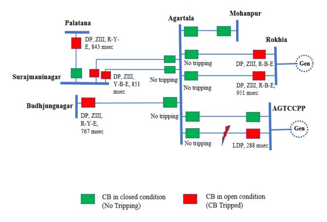
As per DR analysis, double phase to earth fault is in 132 kV AGTCCPP-Agartala II line occurred at 12:34:47.0013 Hrs with Ir=Iy=7 kA, In=5 kA, and Vae=Vbe=18 kV, resulting in a Differential Trip. However, the **circuit breaker (CB) at Agartala did not open**, causing the fault to persist till 12:34:47.836 Hrs. Consequently, the fault was cleared from remote ends of other healthy lines emanating from Agartala on operation of ZIII from Rokhia, Agartala, Budhjungnagar and Palatana.
