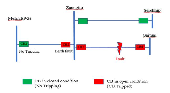
As per FIR submitted by P&ED Mizoram, fault was in 132 kV Zuangtui-Saitual line. Tripping of 132 kV Melriat-Zuangtui line from Zuangtui end for reverse fault in 132 kV Zuangtui-Saitual line is unwanted resulting in blackout of Zuangtui and radially connected substations of Mizoram.
