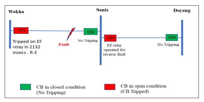
DR of Wokha end of 132kV Sanis-Wokha Line, R-E fault of High resistive nature initiated at 03:54:13.213 Hrs and cleared by Backup EF relay in 2132 msecs at Wokha end. There was no tripping from Sanis end.
