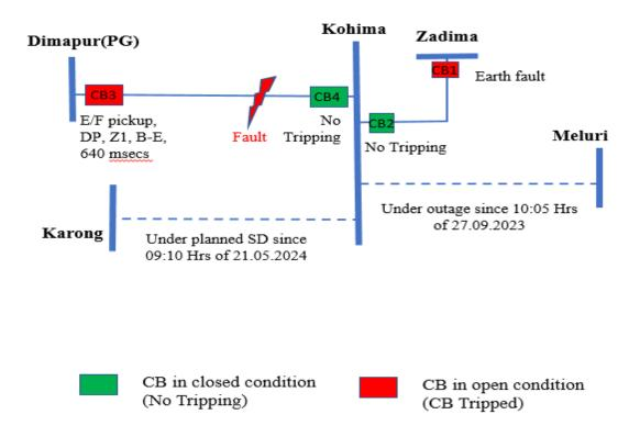
As per DR analysis of 132 kV Dimapur-Kohima line, high resistive B-E fault occurred at 16:42:46.534 Hrs and cleared within 640 msec from Dimapur end. E/F relay pickup at Dimapur end and after around 600 msec, distance protection detected the fault and ZI operated in 40 msec. There was no tripping from Kohima end.
