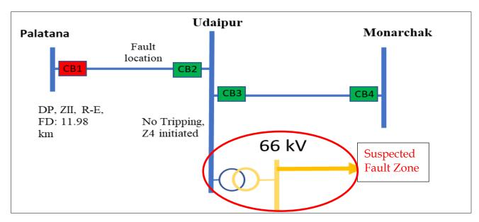
At 07:37 Hrs on 31-03-2024, 132 kV Palatana – Udaipur line tripped at Palatana end on operation of DP, ZII, R-E, FD: 11.98 Km.
