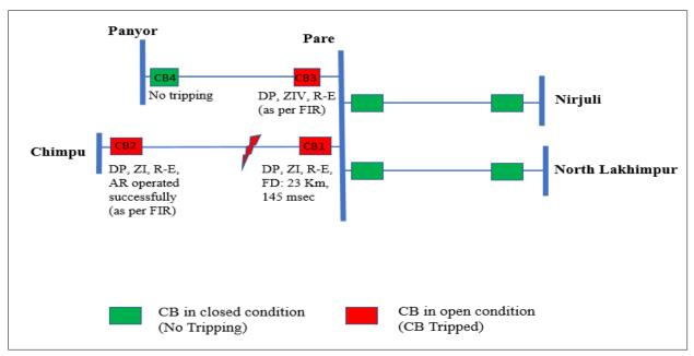
As per DR analysis of 132 kV Pare-Itanagar line, R-E fault initiated at 02:07:24.071 Hrs. After 74 msec, R-phase current increased to 2.9 kA. Fault cleared within 145 msec on operation of DP, ZI (initially ZII pickup) from Pare end.
