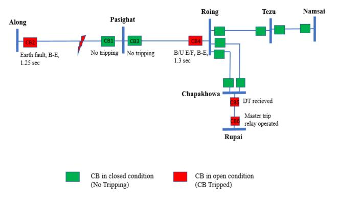
As per DR analysis, resistive B-E fault (Ib-0.32 kA, In-0.26 kA) in 132 kV Along-Pasighat line initiated at 09:24:32.912 Hrs and cleared within 1.25 sec from Along end on operation of directional earth fault. There was no tripping from Pasighat end due to which fault was feeding from Roing end which was finally cleared by tripping of healthy 132 kV Roing-Pasighat line from Roing end (within 1.3 sec) on operation of backup E/F.
