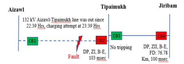
As per DR analysis of 132 kV Jiribam(PG)-Tipaimukh line, solid B-E fault initiated at 23:41:33.831 Hrs and cleared on operation of DP, ZII within 100 msec from Jiribam end.
