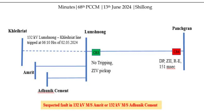
As per DR analysis, R-E fault (Ir-1.8 kA, In-1.4 kA) initiated at 07:00:11.821 Hrs in 132 kV Lumshnong-Panchgram line cleared within 151 msec on operation of DP, ZII from Panchgram end only. ZIV start at Lumshnong end which inferred that fault is in reverse direction.
