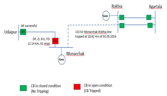
As per DR analysis of 132 kV Monarchak-Udaipur line, B-E fault (Ib-2.4 kA, In-2.6 kA) initiated at 18:32:20.233 Hrs and cleared within 61 msec on operation ZI from Monarchak end. Auto recloser was successful from Udaipur end. Following observations:
