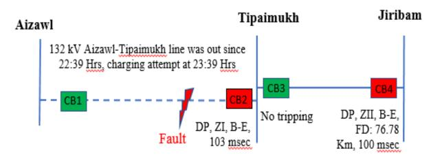
As per DR analysis of 132 kV Jiribam(PG)-Tipaimukh line, solid B-E fault initiated at 23:41:33.831 Hrs and cleared on operation of DP, ZII within 100 msec from Jiribam end.
