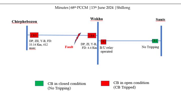
As per DR analysis, Y-B fault occurred at 14:52:50.632 Hrs in 132 kV Wokha-Chiehphebozou line cleared on ZI within 70 msec from Wokha and within 412 msec from Chiephebozou end on ZII.
