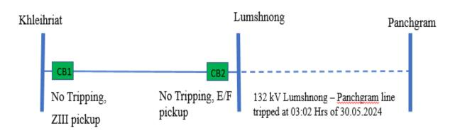
As per DR analysis of Khliehriat end, solid R-Y-B fault (Ir-2.2 kA, Iy-2.4 kA, Ib-2,4 kA) initiated at 06:38:48.098 Hrs and fault current disappeared within 64 msec. Again, at 06:38:48.322 Hrs, Y-E fault (Iy-1.5 kA, In-1.3 kA) reappeared and fault current disappeared within 471 msec. **DP, ZIII** pickup at Khliehriat end. There was no tripping from Khleihriat end.
