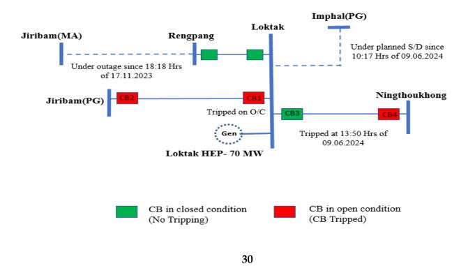
At 13:53 Hrs of 09-06-2024, 132 kV Loktak-Jiribam(PG) Line tripped from Loktak end on Overcurrent which led to tripping of all units of Loktak leading to generation loss of 70 MW.
