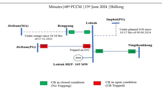
At 10:32 Hrs of 09-06-2024, 132 kV Loktak-Jiribam(PG) line tripped from Loktak end on Overcurrent due to which 132 kV Loktak-Ningthoukhong line got overloaded and subsequently all three units of Loktak tripped leading to generation loss of 105 MW.
