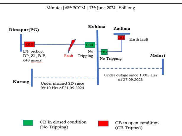
As per DR analysis of 132 kV Dimapur-Kohima line, high resistive B-E fault occurred at 16:42:46.534 Hrs and cleared within 640 msec from Dimapur end. E/F relay pickup at Dimapur end and after around 600 msec, distance protection detected the fault and ZI operated in 40 msec. There was no tripping from Kohima end.
