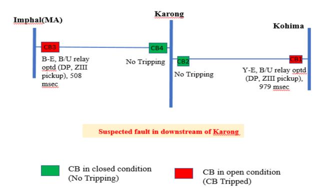
ZIII pickup at Imphal (MA) and Kohima end for 132 kV Imphal(MA)-Karong and 132 kV Karong-Kohima lines clearly indicates that fault was in the downstream of Karong.
