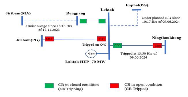
At 13:53 Hrs of 09-06-2024, 132 kV Loktak-Jiribam(PG) Line tripped from Loktak end on Overcurrent which led to tripping of all units of Loktak leading to generation loss of 70 MW.
