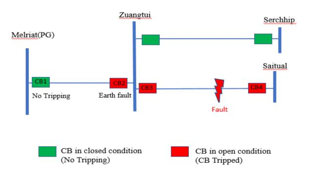
As per FIR submitted by P&ED Mizoram, fault was in 132 kV Zuangtui-Saitual line. Tripping of 132 kV Melriat-Zuangtui line from Zuangtui end for reverse fault in 132 kV Zuangtui-Saitual line is unwanted resulting in blackout of Zuangtui and radially connected substations of Mizoram.
