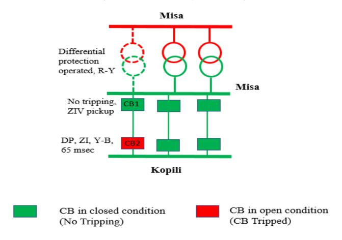
400/220 kV ICT-I at Misa tripped on operation of differential protection.
