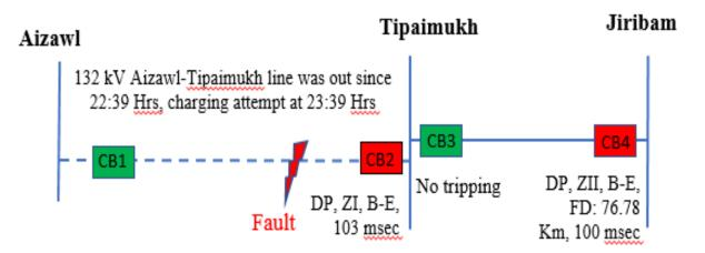
As per DR analysis of 132 kV Jiribam(PG)-Tipaimukh line, solid B-E fault initiated at 23:41:33.831 Hrs and cleared on operation of DP, ZII within 100 msec from Jiribam end.
