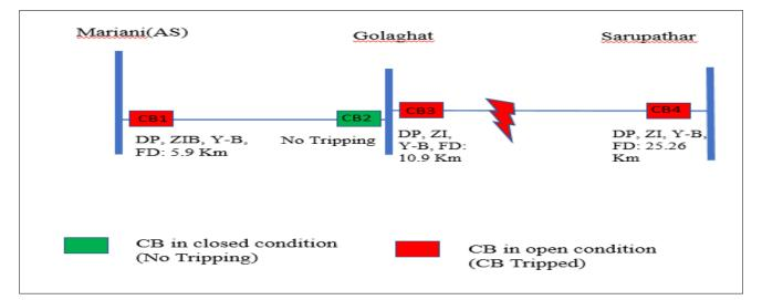
Tripping of 132 kV Golaghat-Mariani (AS) Line from Mariani end on ZI (extended zone) seems unwanted. AEGCL needs to incorporate time delay in ZI (extended zone) protection to avoid unwanted tripping of elements.
