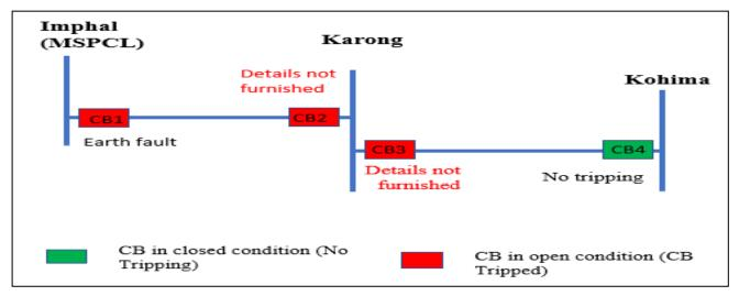
As per the PMU snap of the Imphal SS, Y phase fault with Fault current of 414 A appears in the Y phase and cleared in 80 msec.
