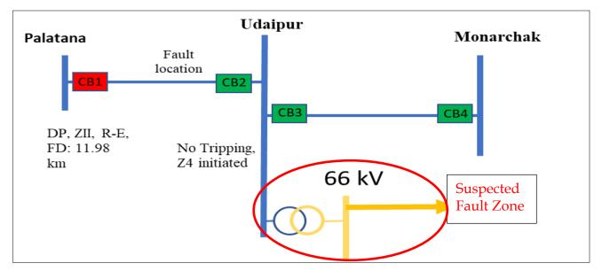
At 07:37 Hrs on 31-03-2024, 132 kV Palatana – Udaipur line tripped at Palatana end on operation of DP, ZII, R-E, FD: 11.98 Km.
