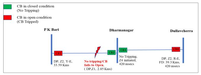
As per DR analysis, R-E fault appears in 132 kV PK Bari – Dharmanagar cleared from P K Bari end only. CB at Dharmanagar, detected in ZI & issued trip command immediately. However, CB fail to open till 420 msecs resulted into ZII tripping at Dullavcherra end.
