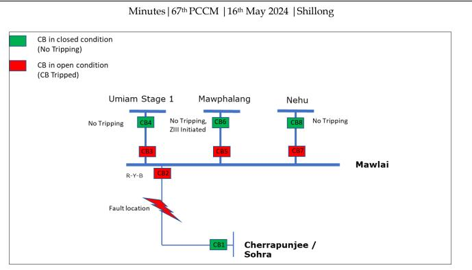
As per DR analysis, R-Y-B phase fault (Ir=Iy=Ib=1.4 kA) initiated at 17:13:24.164 Hrs in 132 kV Mawali- Cherapunji Line which was cleared on operation of DP, ZI within 64 msecs from Mawlai end by opening the CB at Mawlai.
