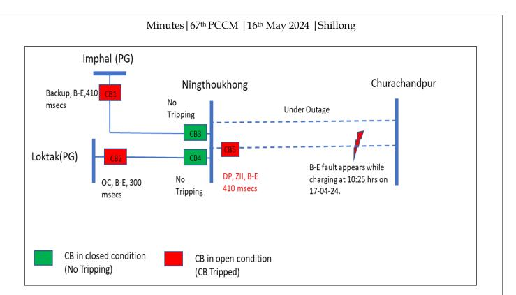
As per DR signal from Ningthoukong, B-E (with Ib:2.5 kA, Vbe:38 kV) solid fault start in 132 kV Ningthoukong-CCpur-2 Line and fault was cleared with Z-II from the system in 410 msecs.
