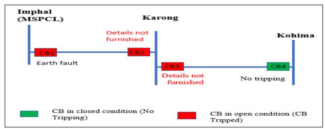
As per the PMU snap of the Imphal SS, Y phase fault with Fault current of 414 A appears in the Y phase and cleared in 80 msec.
