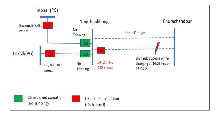
As per DR signal from Ningthoukong, B-E (with Ib:2.5 kA, Vbe:38 kV) solid fault start in 132 kV Ningthoukong-CCpur-2 Line and fault was cleared with Z-II from the system in 410 msecs.
