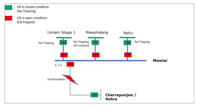
As per DR analysis, R-Y-B phase fault (Ir=Iy=Ib=1.4 kA) initiated at 17:13:24.164 Hrs in 132 kV Mawali- Cherapunji Line which was cleared on operation of DP, ZI within 64 msecs from Mawlai end by opening the CB at Mawlai.
