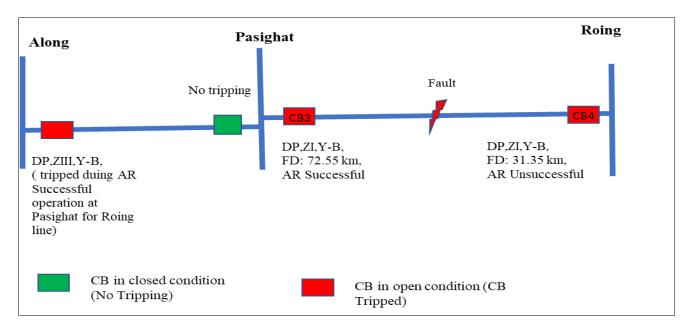
As per DR analysis, Y-B phase fault initiated at 21:55:22.428 Hrs in 132 kV Pasighat- Roing line which was cleared on operation of DP, ZI within 65 msecs & 75 msecs from Pasighat and Roing end.
