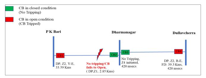
As per DR analysis, R-E fault appears in 132 kV PK Bari – Dharmanagar cleared from P K Bari end only. CB at Dharmanagar, detected in ZI & issued trip command immediately. However, CB fail to open till 420 msecs resulted into ZII tripping at Dullavcherra end.
