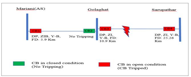
Tripping of 132 kV Golaghat-Mariani(AS) Line from Mariani end on ZI (extended zone) seems unwanted. AEGCL needs to incorporate time delay in ZI (extended zone) protection to avoid unwanted tripping of elements.
