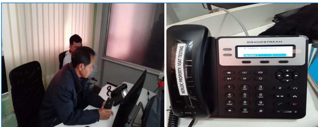
Figure 9: Session Initiated Protocol Phones Installed for Voice Testing under Pilot Project
