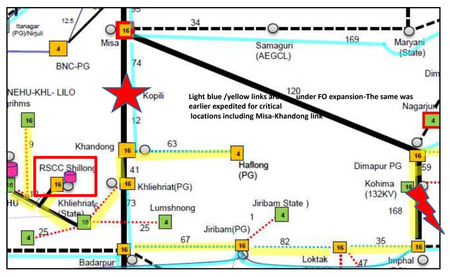
While planning NER FO Expansion project integrated with original ULDC network, team of CTU/POWERGRID, NERTS had selected, some points of fiber bypass (for some nodes) for formation of STM16 ring with Main 1&2 during 17th & 18th NERPC. Accordingly equipments were placed in Misa & Khandong. Based on same, Kopili node could be bypassed in one day time & Misa to Khandong OPGW-1 pair was made running via Fibcom equipment installed under NER FO Expansion.
