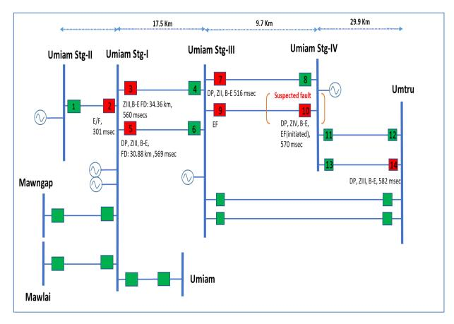
As per DR analysis, 132 kV Umiam Stage 1- Umiam Stage 3 Line 1 & 2 tripped from Umiam Stage 1 end in 560 msecs & 570 msecs respectively on operation of DP, ZIII indicates that fault is beyond the line.
