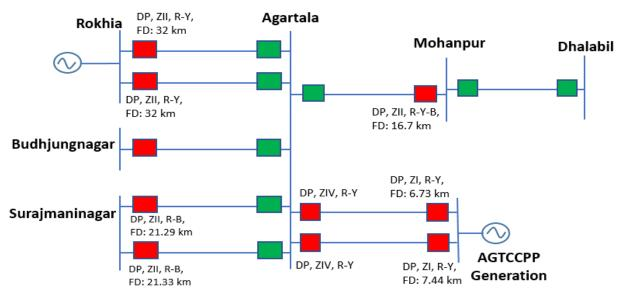
As per preliminary analysis, R-Y fault detected in 132 kV AGTCCPP-Agartala D/C which was cleared on operation of Z-I from AGTCCPP end. As per information from POWERGRID, ZIV was initiated at Agartala end for both the lines which indicates that the fault is in reverse direction of Agartala.
