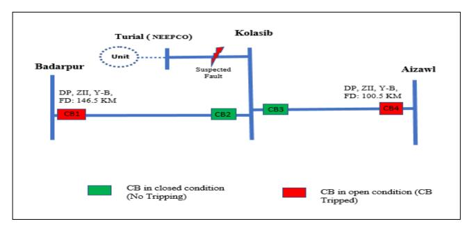
As per DR analysis, Y-B fault detected from Aizawl and Badarpur end which was cleared on operation of DP, ZIII within 850 msec. There was no tripping from Kolasib end for both the lines. Fault is suspected in 132 kV Kolasib-Tuirial line which was not cleared resulting in tripping of healthy 132 kV Aizawl-Kolasib and 132 kV Badarpur-Kolasib lines from remote end on operation of DP, ZIII which impacts the ISTS node
