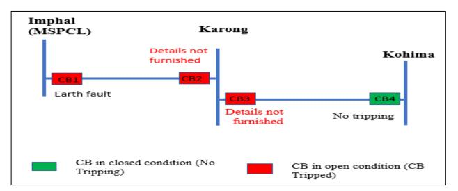
As per the PMU snap of the Imphal SS, Y phase fault with Fault current of 414 A appears in the Y phase and cleared in 80 msec.
