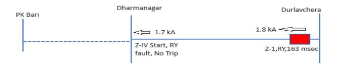
At 11:43 Hrs on **15-09-2023**, 132 kV Dharmanagar – Dullavchera Line tripped from Durlavchera on Z-1 operation within 163 msec. No tripping recorded from Dharmanagar end as it detects fault in Z-IV. It seems that Phase-to-Phase fault was in downstream side of Dharamanagar.
