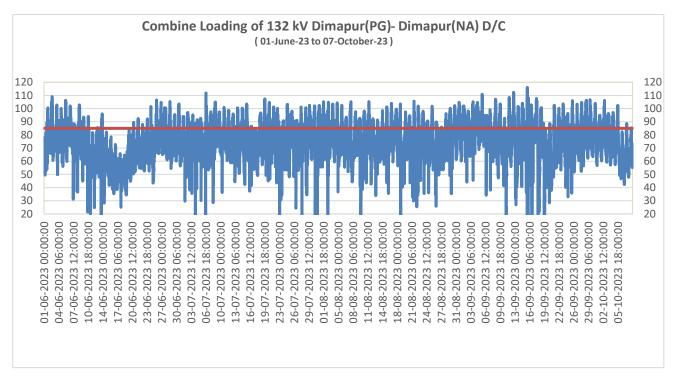
Loading profile of Dimapur shows N-1 contingency of any one circuit not satisfied most of the time as the combine loading was above 85 MW for 22% of times and above 80 MW for 35% of times.
