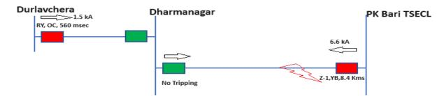
Phase to Phase fault was in 132 kV PK bari-Dharmanagar Line and fault was cleared from PK Bari within 60 msec. Protection system at Dharmanagar **fails to isolate** the fault, due to which fault was feeding continuously from adjacent healthy Line 132 kV Durlavchera-Dharmanagar from Durlavcherra end and finally clear the fault within 560 msec on B/U O/C protection.
