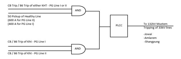
Fig: SPS Schematics at 132kV Khliehriat S/S for 132kV PG Line I & II
