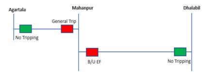
At 02:33 Hrs on 29-Sept-2023 both 132 kV Agartala- Monahpur Line & 132 kV Dhalabil - Mohanpur line tripped from the **Mohanpur end** on operation **Earth Fault** and **General Trip which led to blackout of Mahanpur Substation**. No tripping was observed from the other end such as Agartala & Dhalabil.
