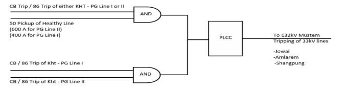
Fig: SPS Schematics at 132kV Khliehriat S/S for 132kV PG Line I & II
