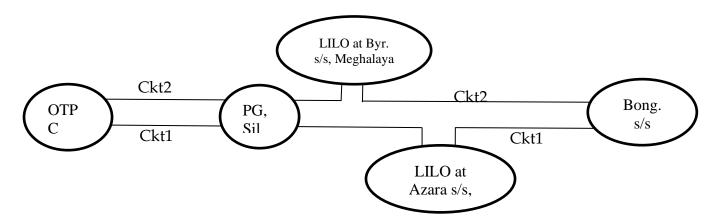
During the last financial year (FY 2022-23), there were instances of tripping in the 400 kV D/C Palatana-Bongaigaon Transmission System. Due to inaccurate fault calculations of the relays, difficulties were faced in detection of fault location. In normal scenarios, we expect to locate the faults within a range of +/-5 km from the relay distance measurement. However, during post-fault patrolling, we discovered fault locations approximately 10-15 km away from the relay's calculated distance.
