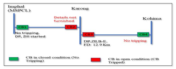
As per DR analysis of karong end, High resistive vegetation fault in 132 kV Karong – Kohima line with fault current increasing gradually upto 1 kA and phase voltage reduces to 47 kV.
