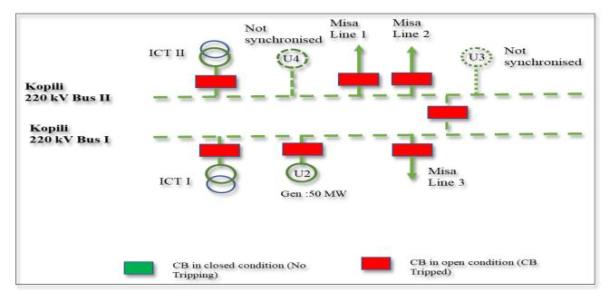
**Summary:** LBB protection operated at 220 kV Kopili Bus I & II and DT received at Misa end leads to the generation loss of 50 MW.
