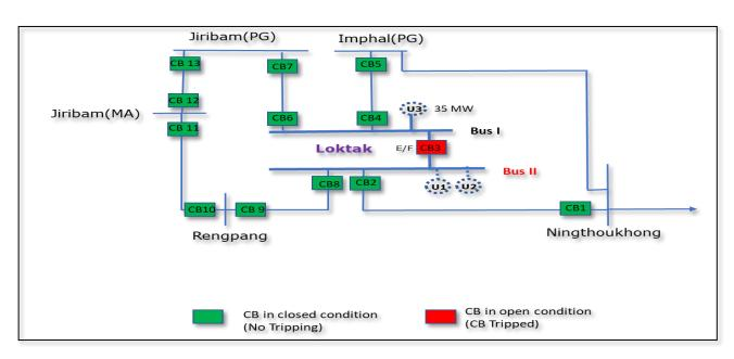
The blackout of Bus II at Loktak observed in the 3 occasions due to the tripping of Bus Coupler at Loktak are listed below:
