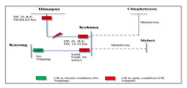
As per DR analysis, Metallic fault in 132 kV Dimapur (PG) – Kohima line successfully cleared from the Kohima end in 77 msecs on operation of DP, ZI, B-E, FD: 12.53 km. Fault current of 940 A observed in neutral.
