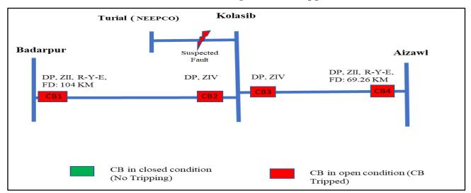
Tripping at Badarpur & Aizawl end on ZII and tripping of both the line at Kolasib end on ZIV indicates the fault in the downstream of Kolasib substation.
