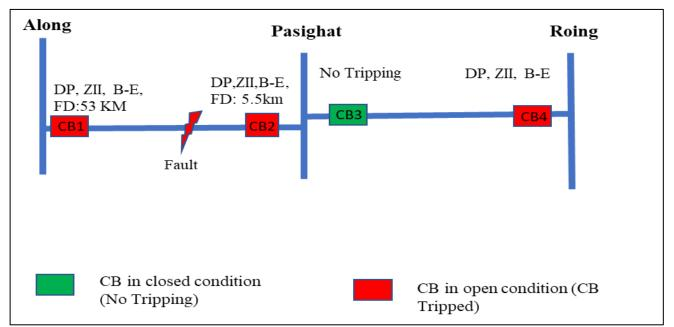
Fault at a distance 5.5 KM from the Pasighat end cleared on operation of DP, ZII from Along & Pasighat end in 623 msecs & 557 msecs. Also, 132 kV Pasighat – Roing tripped at Roing end in 547 msecs leading to the blackout of Pasighat substation of the Arunachal Pradesh power system.
