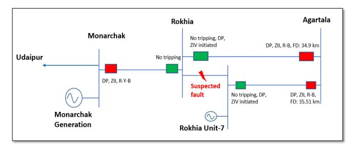
As per DR analysis, suspected fault is suspected in 132 kV Rokhia-Rokhia link feeder which was cleared by tripping of 132 kV Rokhia-Agartala D/C & 132 kV Monarchak-Rokhia lines from remote end on operation of Z-II. Also, ZIV initiated at Rokhia end for 132 kV Rokhia-Agartala D/C & 132 kV Rokhia-Monarchak lines indicates that fault is in reverse direction.
