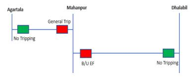
At 02:33 Hrs on 29-Sept-2023, both 132 kV Agartala- Mohanpur Line & 132 kV Dhalabil - Mohanpur line tripped from the **Mohanpur end** on operation of **Earth Fault** and **General Trip which led to blackout of Mohanpur Substation**. No tripping was observed from the other end such as Agartala & Dhalabil.
