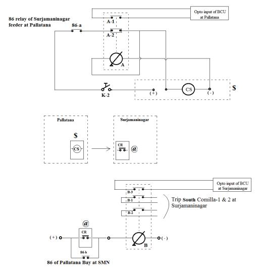
Alternatively Pallatana may send Direct Trip command to Surjamaninagar in case of three phase trippng
