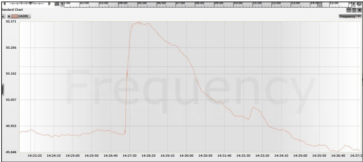
Fig 2: Frequency Plot where frequency shoot up to 50.37 Hz and revived within six minutes
