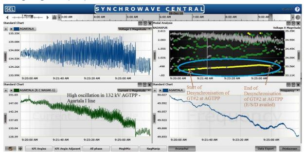
On 03<sup>rd</sup> January'17 from 07:43 Hrs onwards, oscillation was seen prominently in Voltage, at 132 kV Agartala PMU for a long duration of around 3 Hours.
