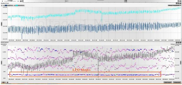
On 10<sup>th</sup> January'17 from 22:04 Hrs onwards, oscillation was seen prominently in Voltage, at 132 kV Agartala PMU.
