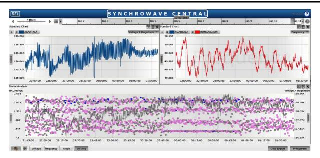
On 11<sup>th</sup> January'17 from 23:23 Hrs onwards, oscillation was seen prominently in Voltage, at 132 kV Agartala PMU.
