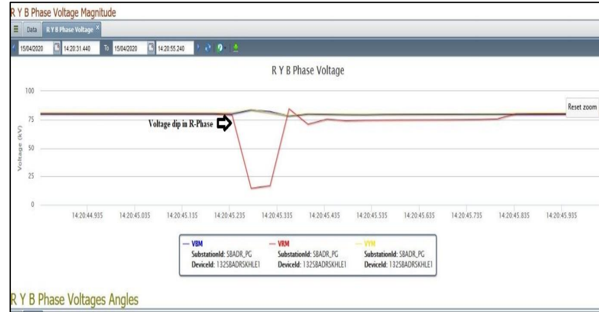
Figure-1: PMU Voltage Signal of 132 kV Badarpur-Khliehriat
